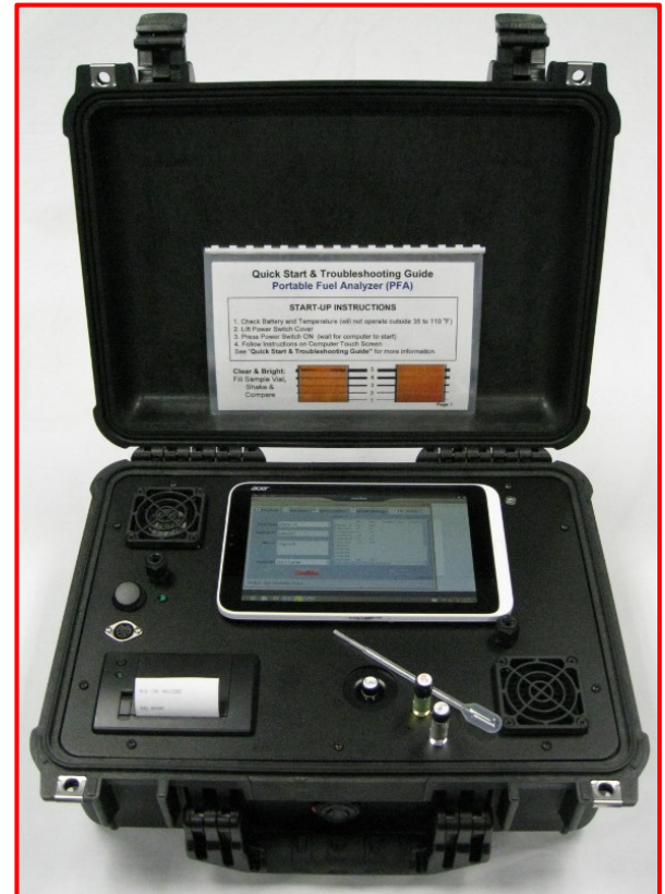
Portable Fuel Quality Analyzer 7x13x16", 14 lbs.
